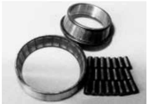
Fig. 15-12 Corrosion on Tapered Roller Bearing
