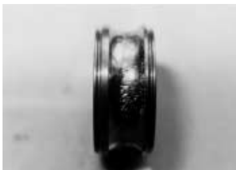
Fig. 15-1 Generation of Flaking on Inner Ring Raceway of Deep Groove Ball Bearing
