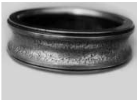
Fig. 15-2 Generation of Flaking on Inner Ring Raceway of Deep Groove Bearing
